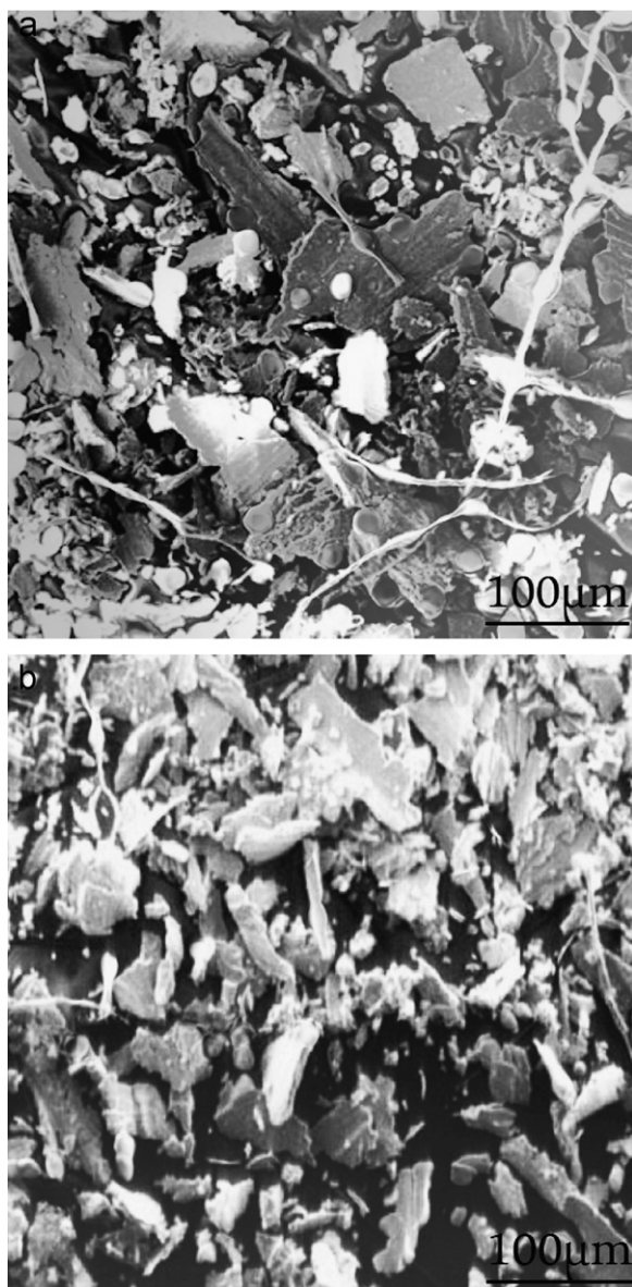
Fig. 9. The worn debris of: (a) base Al alloy and (b) the composite.
