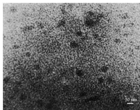
Fig. 3. Transmission electron micrograph of glass–ceramic sample heated at 620 °C for 10 h.
