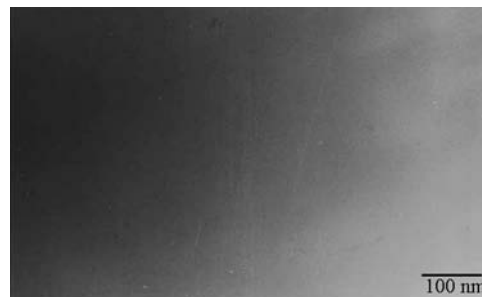
Fig. 2. Transmission electron micrograph of as-annealed glass-sample.
