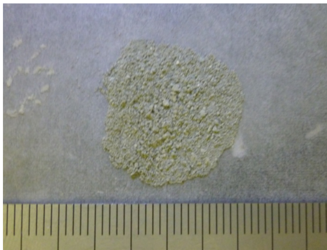
Fig. 2. Appearance of recovered powder in experiment in air atmosphere.
