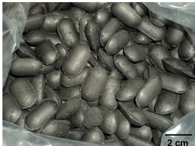
Fig. 1. Prepared briquettes containing a mixture of spent MgO–C bricks, dolomite fines, iron scales, coke and a natural binder (linseed oil). The briquette length is 25.4 mm (~1 in.).
