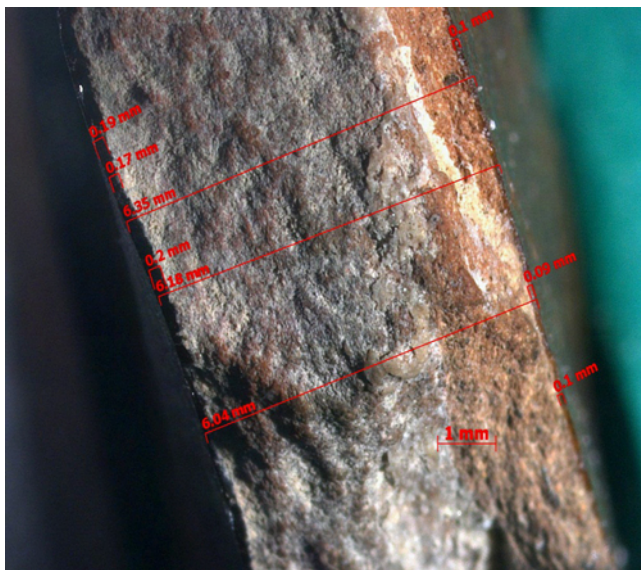
Fig. 4. Cross section of sherd C5 with measurement of thickness of sherd and glaze.
