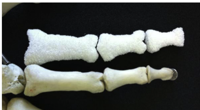
Fig. 9. Scaffold of finger using PU template coating method by HA slurry.
