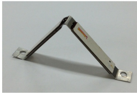
Fig. 7. Fabricated stator (ceramic and elastic body).
