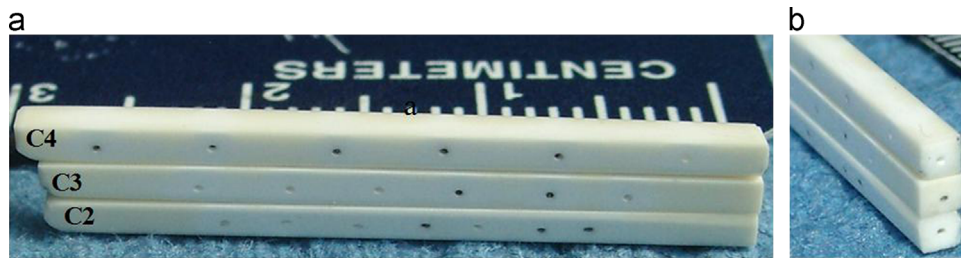
Fig. 1. Specimen C series containing 373 \mu\text{m} diameter channels. The specimens C1, C2 and C3 are stacked to show the relative spacing of the channels: (a) side view showing several channels normal to the span; and (b) end view showing single channel along each specimen span.
