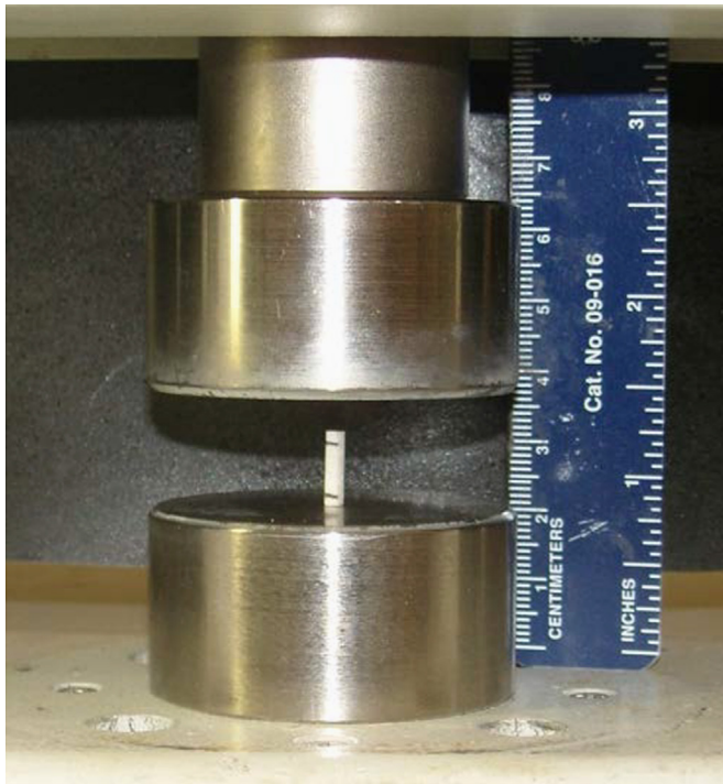
Fig. 2. Set-up for compression test showing compression specimen between platens.
