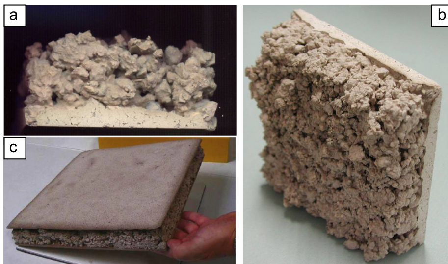
Fig. 8. Pictures of the material scale up: sample dimensions vary from 5 cm × 5 cm × 2.5 cm (a) to 15 cm × 15 cm × 3.5 cm (b) and finally 30 cm × 30 cm sandwich panel (c) was prepared with 0.5 cm thick skins of composition B and 4 cm thick core of composition L (see Table 1).
