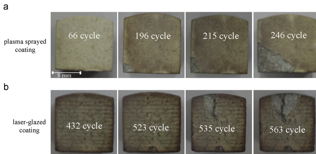
Fig. 6. Macroscopic image of: (a) plasma-sprayed and (b) laser-glazed samples during thermal shock testing.
