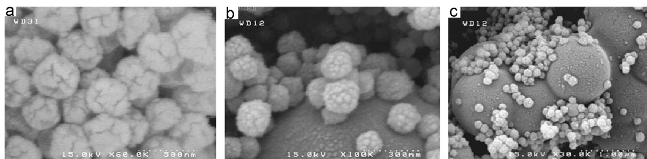
Fig. 10. SEM images of the as-prepared \alpha -Fe 2 O 3 samples prepared in absence of sodium acetate at (a) 140 °C, 24 h (b) 160 °C, 18 h (c) 180 °C 18 h.
