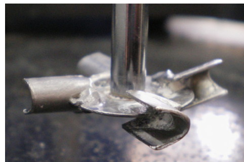
Fig. 2. Image of the turbine-style impeller mixer with four asymmetric concave blades used to create foam.
