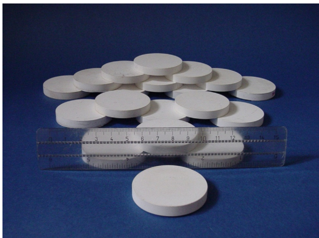
Fig. 1. Porous ceramic aerostatic structures produced using the starch consolidation technique.
