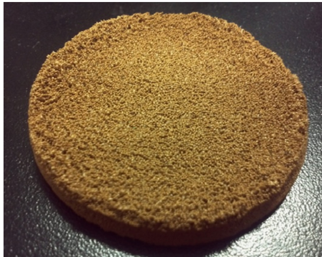
Fig. 2. Stack of porogens heat treated between the pair of glasses at 230 °C for 2 h.
