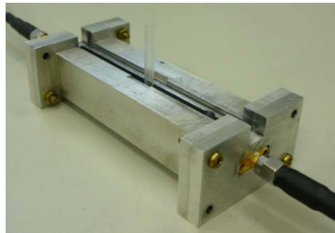
Fig. 1. Photograph of an X-band rectangular resonant cavity for measurement of complex permittivity and permeability of microwave absorbing composites.
