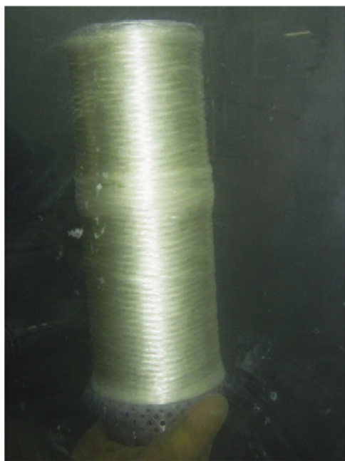
Fig. 5. The filament bobbin of the N -methylpolyborosilazane green fibres.
