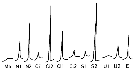
Fig. 2. DTA 970°C exotherms of the powders studied.
