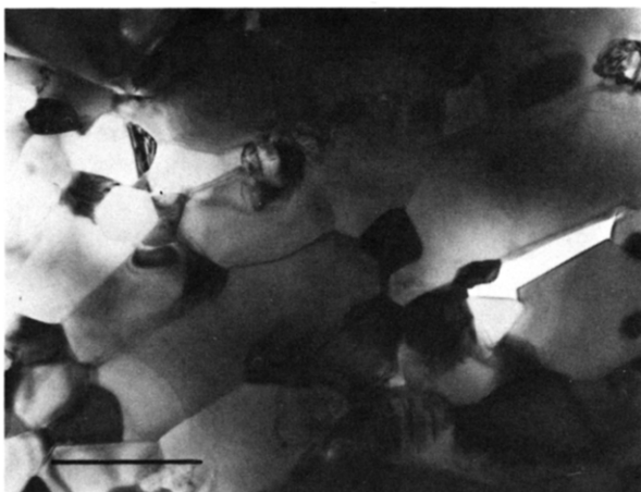
Fig. 5. Electron micrograph of S\perp specimen strained up to 88% at 1400°C under 50 MPa; the arrow is parallel to the compression axis. Scale bar = 1 \mu m.
