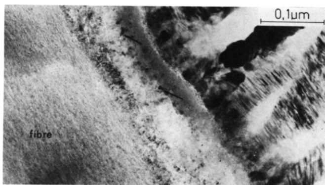
Fig. 9. Graphite particles (indicated by arrows) in the carbon layer of a C-fibre composite after three-point bending at 1300°C under vacuum.
