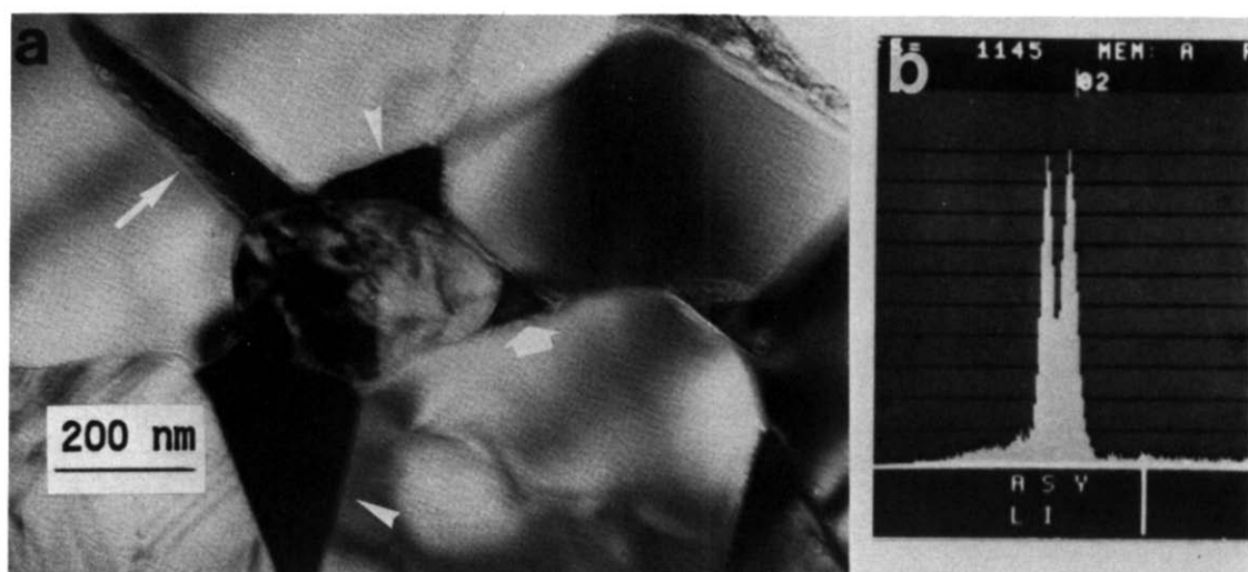
Fig. 5. Identification and localization of the Y2S by TEM and EDS. (a) Bright-field showing different Y2S grains (different arrows) formed by devitrification at 1523 K of the glassy interphase; (b) EDS spectrum.
