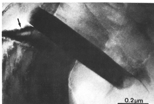
Fig. 3. Transmission electron micrograph. Bright field sample A quenched from 900^\circ\text{C} . Rod of \text{Bi}_4\text{Ti}_3\text{O}_{12} and an unidentified intergranular phase ( \rightarrow ).
