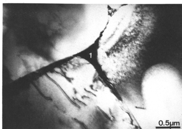
Fig. 7. Transmission electron micrograph. Bright field sample A quenched from 1100^\circ\text{C} . ZnO grains with dislocations. Unidentified intergranular phase (1).
