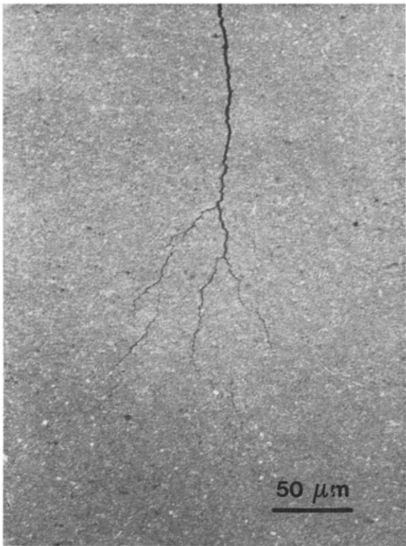
Fig. 3. Optical micrograph of a crack in a testbar loaded to K^*_{IC} = 15 \text{ MPa}\sqrt{\text{m}} in vacuum at 1320°C and unloaded before final failure. The overall appearance of the crack, dominated by crack branching and microcracks is shown.
