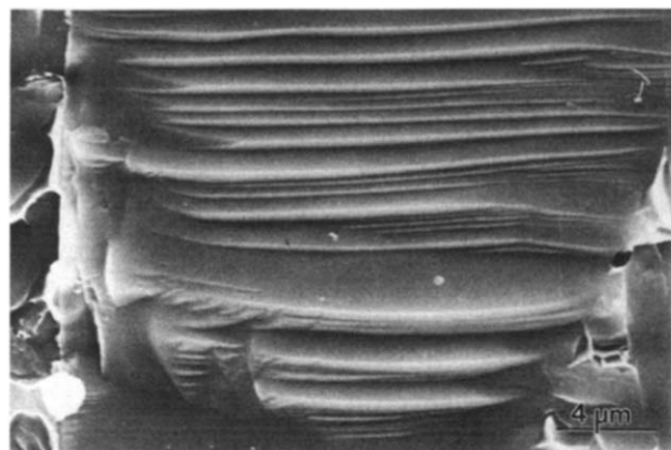
Fig. 10. Example for stepwise cleavage fracture provides hint for possible existence of elastic bridges (FGS composite).
