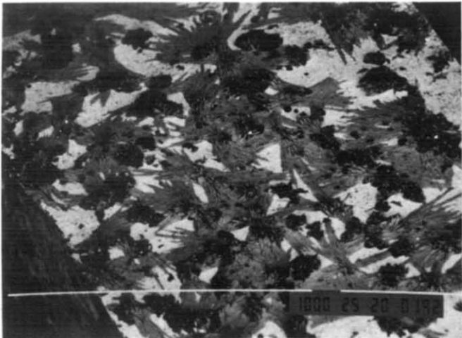
Fig. 7. Surface of \text{La}_{0.6}\text{Ca}_{0.4}\text{Cr}_{0.9}\text{Ni}_{0.1}\text{O}_3 quenched from 1170°C during sintering. Backscattered electron image. Magnification \times 75 ; bar, 1000 \mu\text{m} .
