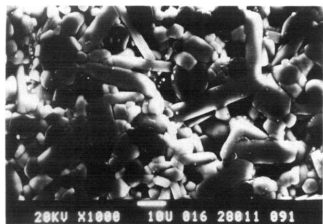
Fig. 5. Microstructure of Nb-containing RBAO showing needle-like grains formed in situ after aging at 1400°C for 24 h. 18
