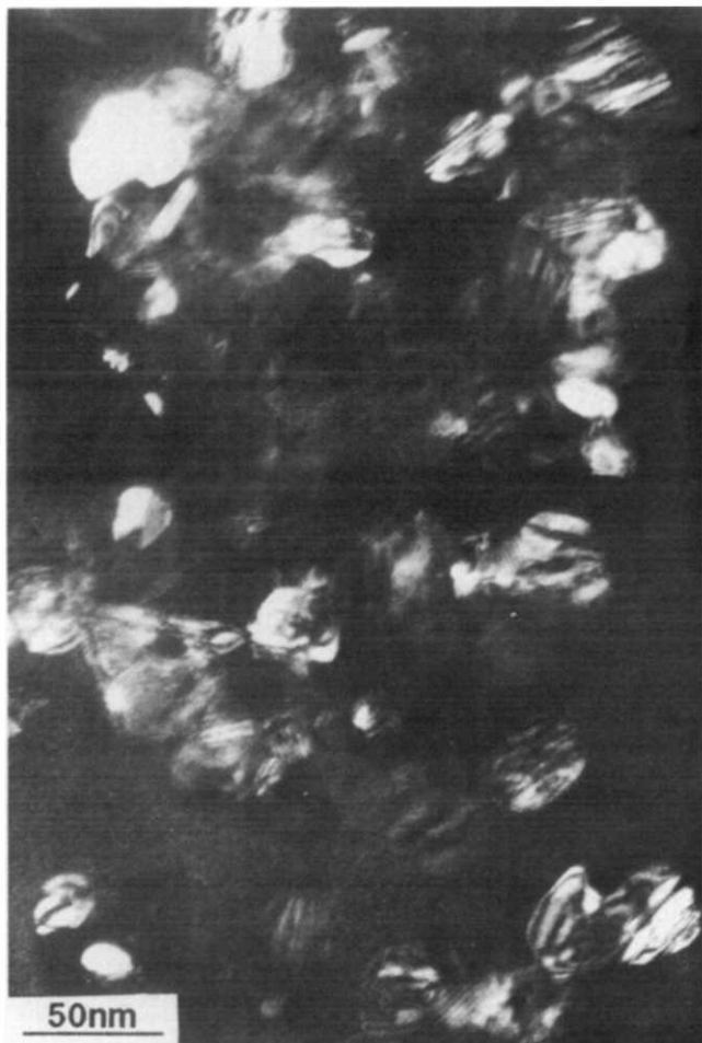
Fig. 13. Position 2 dark field image of part of the fiber (cross-section) for T_p = 1600^\circ\text{C} . Crystals are SiC.
