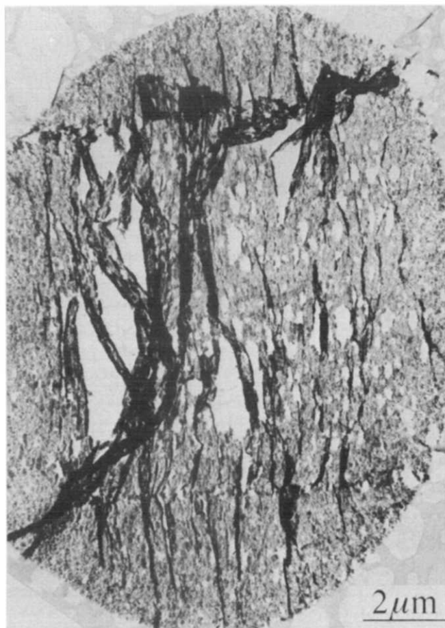
Fig. 15. Experiments under nitrogen. Overall view of the cross-section of the fiber. T_p = 1600^\circ\text{C} . The skin/core effect is no longer visible.
