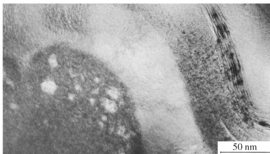
Fig. 9. Interlayer sequence surrounding a surface bay (bottom left) of the fibre.
