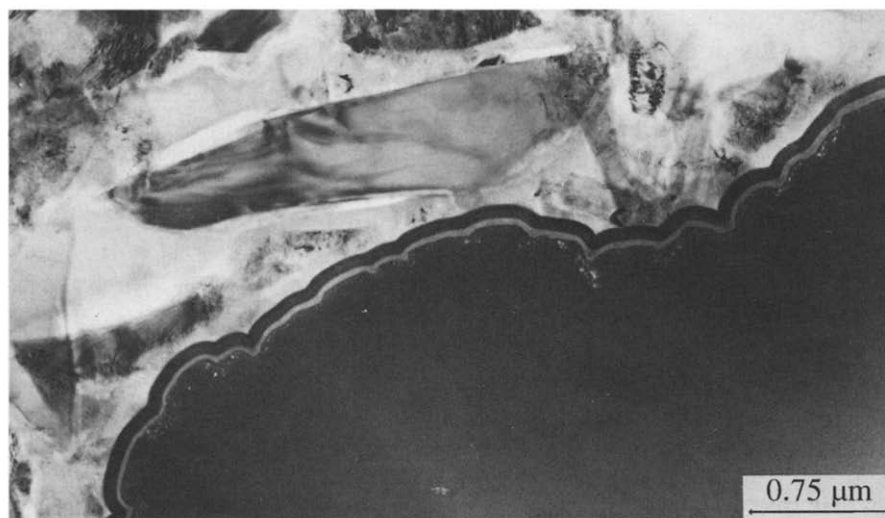
Fig. 6. HVEM image of the interlayer between fibre (bottom) and matrix (top).
