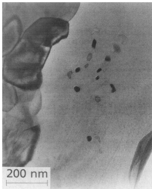
Fig. 3. Mullite crystals formed in the bulk of the silica-rich melt ( T = 1500^\circ\text{C} )
