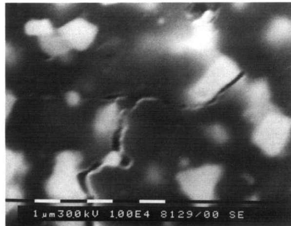
Fig. 6. SEM micrograph showing a crack propagation in SiC-Si-WC sample.
