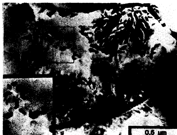
Fig. 7. BF micrograph of the dendritic growth of cordierite in a highly transformed \beta -quartz ss crystal. Orientation of cordierite is [001] parallel to the electron beam. {100} faces are preferentially formed. Heat treatment: 1150°C, 60 min.
