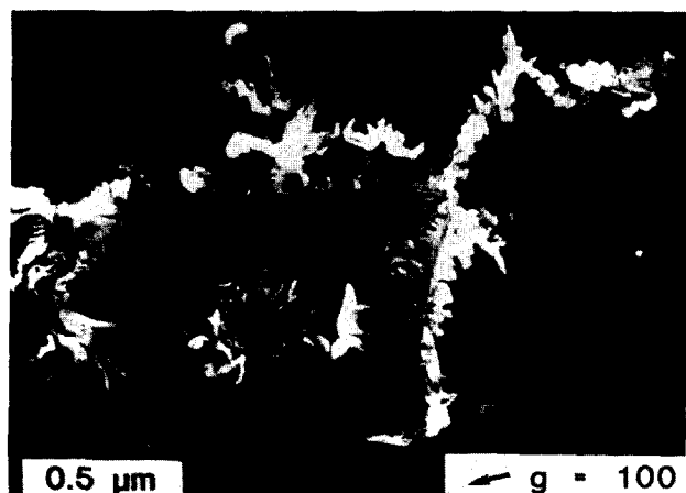
Fig. 5. TEM (100) DF micrograph of the spinal morphology of the cordierite rims on the \beta -quartz ss grain boundaries. Heat treatment: 1150°C, 60 min.
