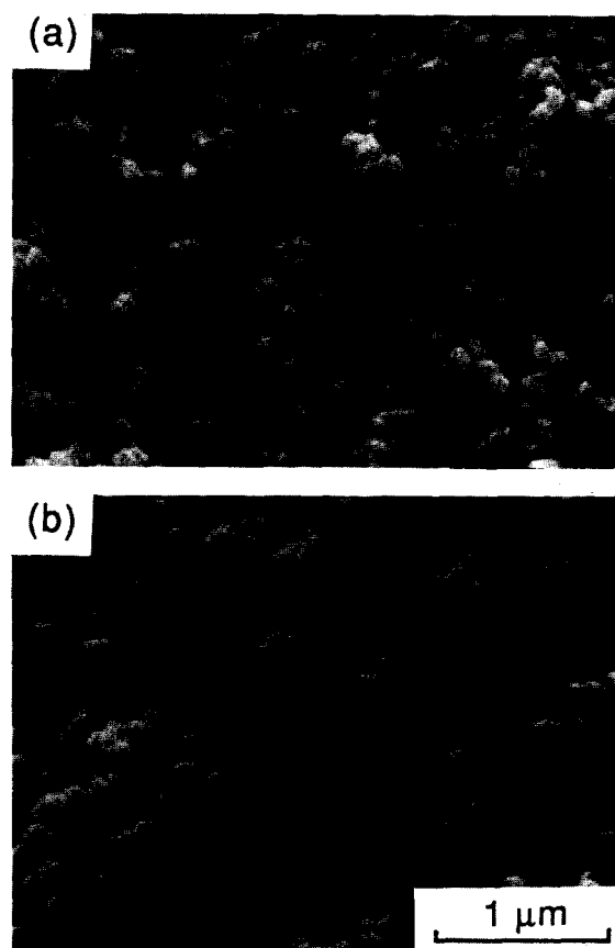
Fig. 5. Scanning electron micrographs of fracture surfaces of TA powder compacts: (a) as compacted, (b) pre-treated at 920°C for 50 h.
