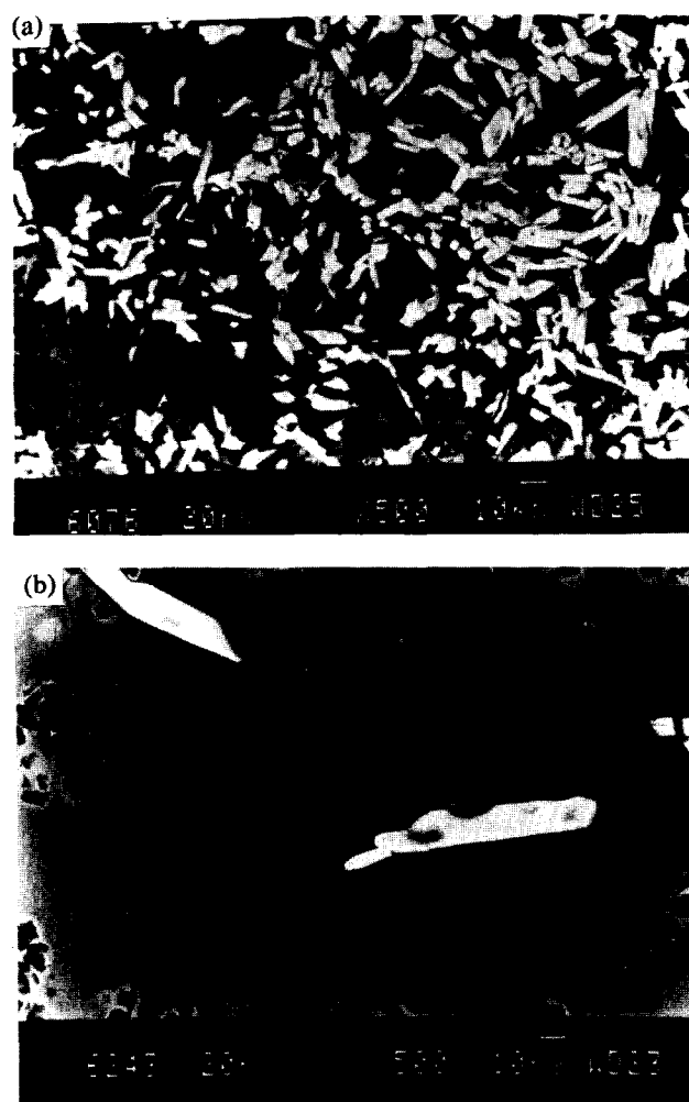
Fig. 8. Surface morphology of 0.5 sialon material after 48 h exposure at 1350^\circ\text{C} in (a) laboratory air environment and (b) simulated flue gas environment.
