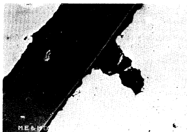
Fig. 7. Lead zirconium titanate ceramic joined using a 5 \mu\text{m} thick aluminium foil.
