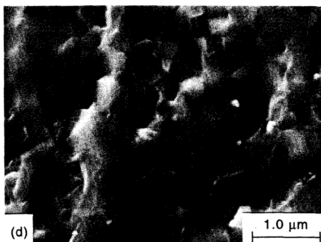
Fig. 12. SEM of the fracture surfaces of the \text{CeO}_2 powder compacts doped with 6 at% of (a) \text{Mg}^{2+} , (b) \text{Ca}^{2+} , (c) \text{Y}^{3+} and (d) \text{Nd}^{3+} after sintering at 10^\circ\text{C}/\text{min} to 1350^\circ\text{C} .
