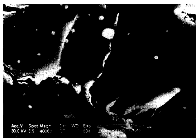
Fig. 9. Cracks formed by coalescence of cavities developed at the surroundings of zirconia particles at grain boundaries during plastic deformation.
