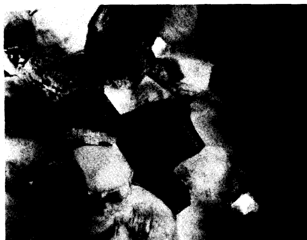
Fig. 6. Microstructure inside the zirconia matrix after a strain of 40% at 1300°C for a specimen pressed at 1550°C. Scale bar = 0.5 \mu\text{m} .
