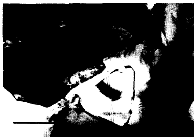
Fig. 7. Crack at a matrix-whisker interface in an extruded sample deformed at 1330°C up to a strain of 34%. The arrow is parallel to the compression axis. Scale bar = 0.5 \mu\text{m} .
