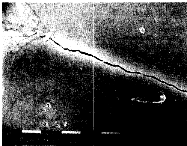
Fig. 6. SEM micrograph showing the crack propagation in SN sample.
