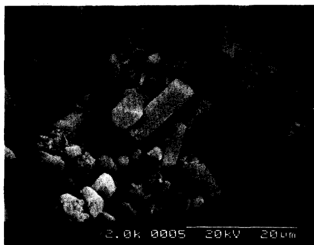
Fig. 5. SEM micrograph showing \beta - \text{Si}_3\text{N}_4 formation in zone close to an intermetallic particle.
