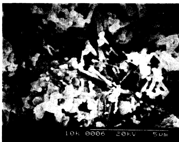
Fig. 4. SEM micrograph showing \alpha -whiskers formed in macropores.
