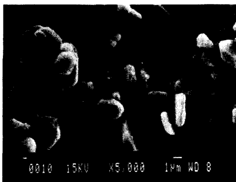
Fig. 7. SEM micrograph of the coarse \alpha - \text{Al}_2\text{O}_3 raw material.
