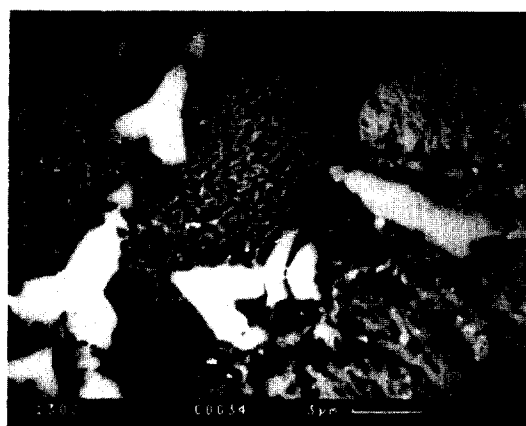
Fig. 10. Crystallization of glass B (1300°C for 1 h). Zr-rich droplets in an area that was originally \gamma - \text{Y}_2\text{Si}_2\text{O}_7 fibres with the interfibrillar glass phase (backscatter image—5000 ×).
