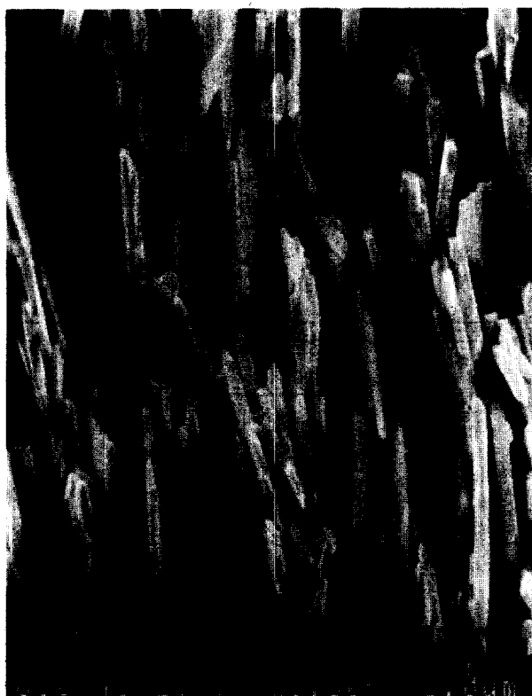
Fig. 6. SEM micrograph of hot-forged \text{PbBi}_8\text{Ti}_7\text{O}_{27} ( \perp to the forging direction)
