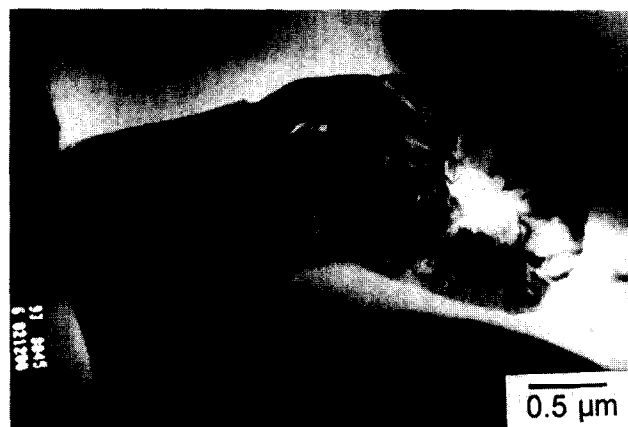
Fig. 4. Transmission electron micrograph of ultra-rapidly quenched mullite glass showing a large residual quartz crystal embedded in a glassy matrix.
