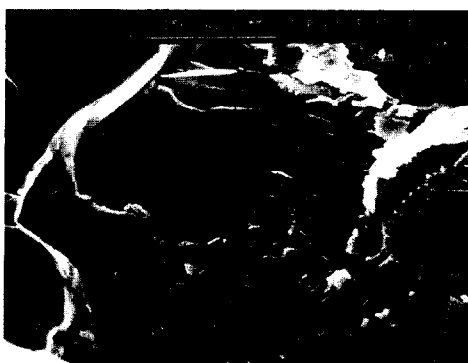
Fig. 2. SEM image of a BaTiO 3 ceramic damaged by 100 shots at 3.2 \times 10^7 W/cm 2 . The ceramic is ablated to a depth of 4–5 \mu m.
