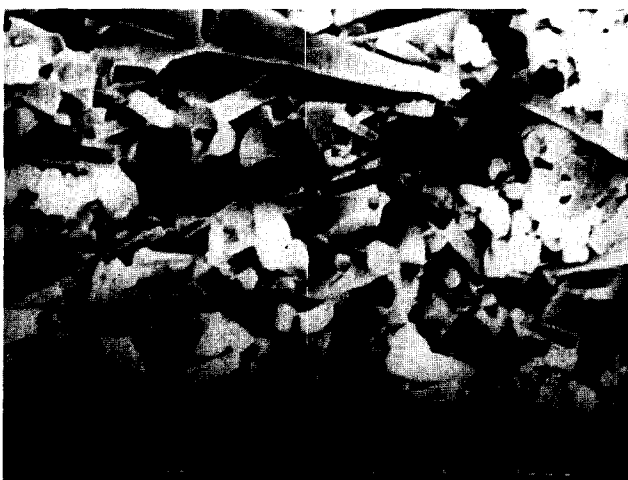
Fig. 10. At high \Delta K region, the alumina grains failed in a mixed mode, i.e. intergranular (~45%) and transgranular (~55%).
