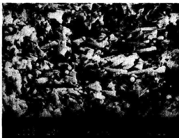
Fig. 7. At high \Delta K (2.8–3 MPa \sqrt{m} ) region the whiskers failed in a mixed mode, i.e. both with a square fracture and also by pullout.
