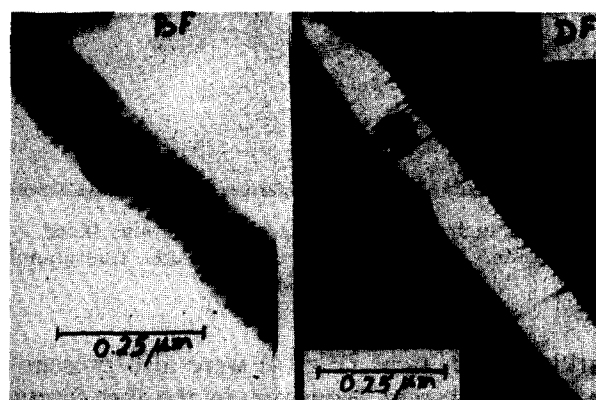
Fig. 15. TEM of \beta -SiC whisker showing stacking fault by dark field and bright field techniques.
