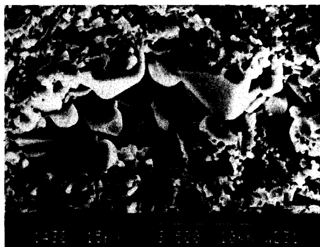
Fig. 2. Fracture surface of the composite showing the size and shape of the alumina matrix.
