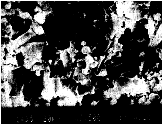
Fig. 9. At low \Delta K region, the alumina matrix failed predominantly through transgranular fracture.
