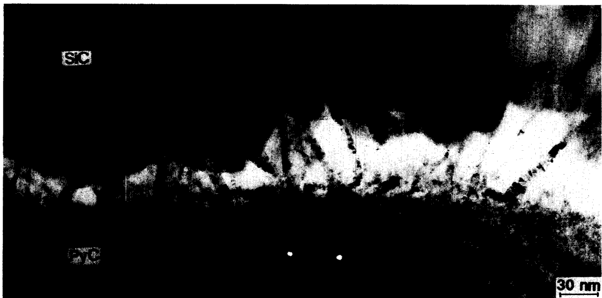
Fig. 18. BF TEM image of a carbon wall area. Note the high porosity.
