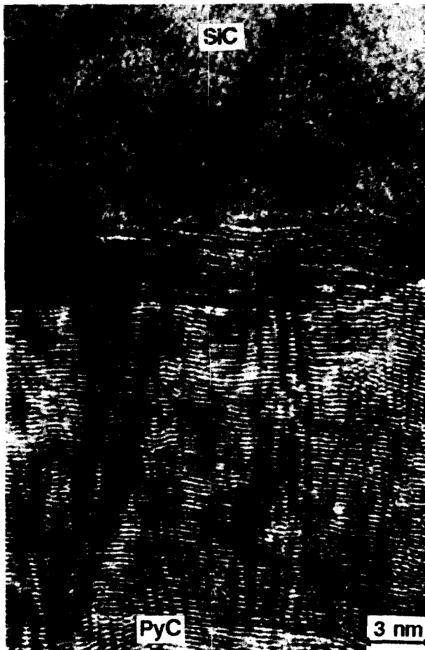
Fig. 13. LF TEM image of the pyrolytic carbon interphase (ANI-PyC) matrix interface. Note the high anisotropy parallel to the interface, and the nearly perfect organisation of the graphene sheets.
