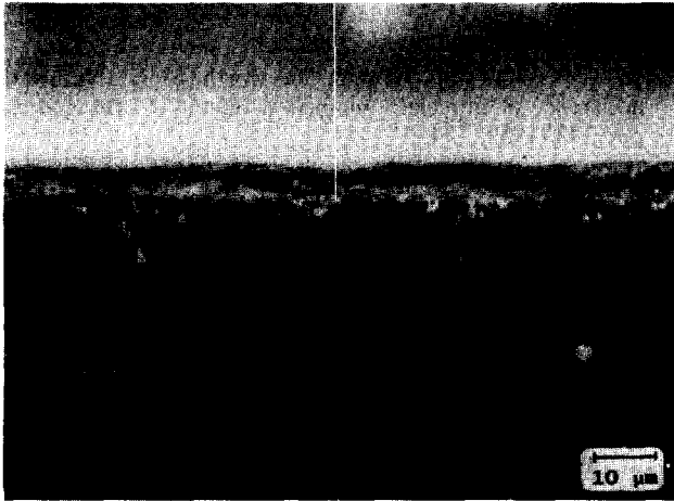
Fig. 4. Micrograph of a kovar/glass interface.
