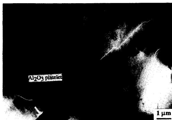
Fig. 8. TEM micrograph of X-sialon matrix composite with 28 vol.% \text{Al}_2\text{O}_3 platelets showing a crack following the X-sialon matrix– \text{Al}_2\text{O}_3 platelets interface. The arrow marks the point where the crack is deflected into the interface. Further along the interface, this crack is not always seen edge-on.
