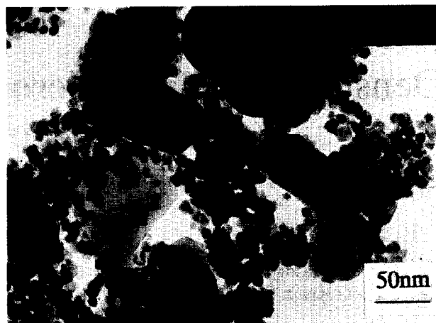
Fig. 1. TEM micrograph of mixed \text{Al}_2\text{O}_3/\text{Y-TZP} composite powder.
