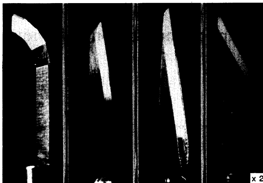
Fig. 1. Experimental samples of surgical knives with blade sharpening radii equal to 0.2–0.5 \mu\text{m} , made of the zirconia crystals studied. They were tested in clinics of Kiev, Moscow and Sydney ( \times 2 ).
