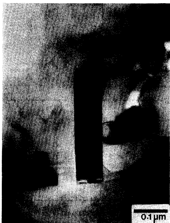
Fig. 9. Transmission electron micrographs showing the preferred nucleation and growth of elongated O'-sialon crystals from the surfaces of SiC grains.
