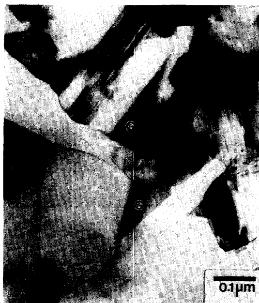
Fig. 6. Representative transmission electron micrograph of microstructure of the composite matrix, showing discrete pockets of glassy phase (G) at three and four grain junctions.
