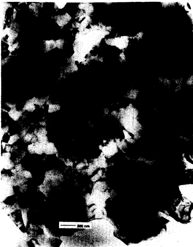
Fig. 2. TEM of 50/50 solid solution alloy of SiC/AlN showing the sub-micron grain size, \approx 1/2 \mu\text{m} .
